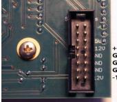
Jomox ModBase 09/ModBrane 11 euro rack supply connector. Please connect the power supply of the eurorack system bus *here*.
