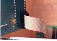
Connect the other end of the ribbon cable to the module as shown on the picture. The cables are fairly short which is good in electrical means to the relatively high power consumption of the module.
