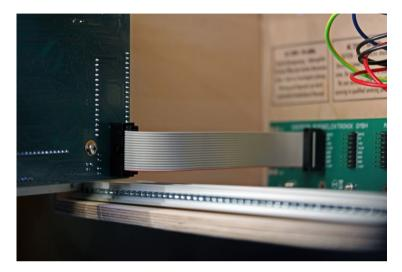
Don't flip the cable but connect it as shown on the picture.
