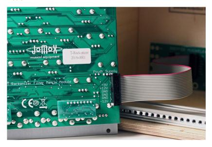
Attention: DO NOT connect, under any circumstances, the power supply cable to the Jomox Inter-D-module bus!!! The rack power supply and the module could get seriously damadged!
