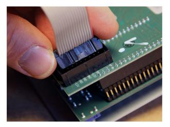
Now connect the module with the reversed cable to the system bus and it will work. No worry, the Jomox module has protection diodes so it will not get damadged. Sorry for your inconveniencies!
