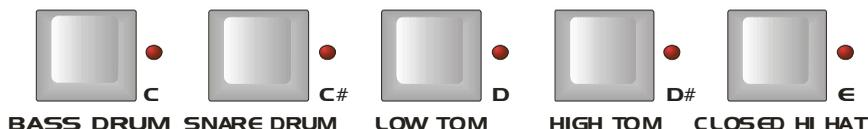
With the **(Instrument)** keys you can select the instrument track to be edited. Each instrument has its own track and its own step programming. Of course you can switch between these whilst the sequencer is running. The 16 **(Step)** LEDs above the buttons indicate on which steps the selected instrument is played (the playing LEDs light up red).
