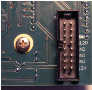
Jomox ModBase09/ModBrane11 euro rack supply connector. Please connect the power supply of the eurorack system bus *here*.
