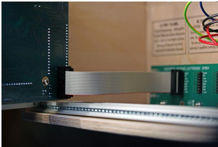
Then please mount the module on the rack rails with the supplied metric M3 screws. In case you want to connect a midi cable, please do this beforehand of mounting.
